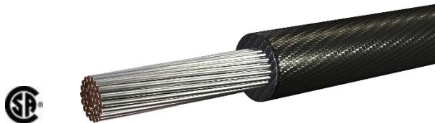
Stranded tinned, annealed copper conductors, extruded silicone rubber insulation, a fiberglass braid jacket is applied over the insulation and treated with high temperature lacquer finish. 200°C, 600 Volts.
