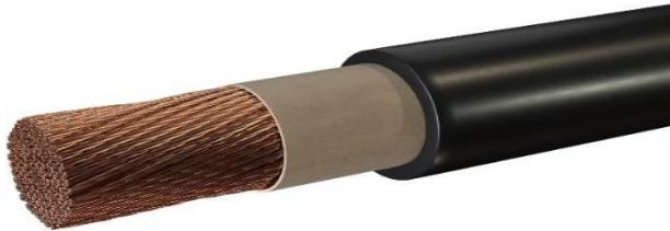
Conductors Flexible stranded bare copper per ASTM B 172 Class K. Separator Paper tape separator between conductor and insulation, Ethylene-propylene rubber (EPR insulation) 600v.
